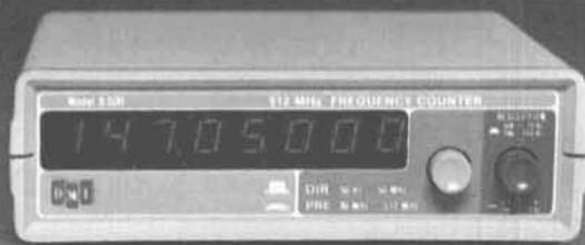
512 MHz FREQUENCY COUNTER 5W X 5 X 1 1/2 50 Hz to 512 MHz 1 PPM ACCURACY TCXO
